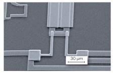
Maskless lithography enables multi-dimensional overlay control beyond standard zoom lens scaling. The Maskless Aligner technology includes compensations for individually scaling x and y directions, rotation, as well as shearing. This capability is demonstrated with an 18-layer SQUID device which shows excellent overlay through all layers (exposure here on MLA 150).
