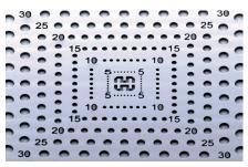
The surface of ceramic substrates as are used in the production of electronic components may have local thickness variations. The MLA 300 real-time auto focus follows these variations, leading to a superior uniformity of the resulting design.
