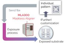
The benefit of Maskless Lithography is the inherent rapid turnaround and adaptation of the exposed patterns. Modifications for customized products no longer entail production and maintenance of an expensive mask set. Switching between product types is seamless, and does not require intervention to change masks.
